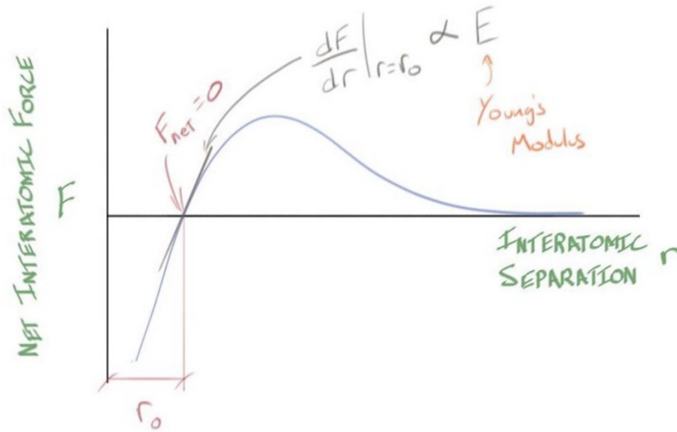
Figure 10: Interatomic force versus interatomic separation curve for two hypothetical atoms
